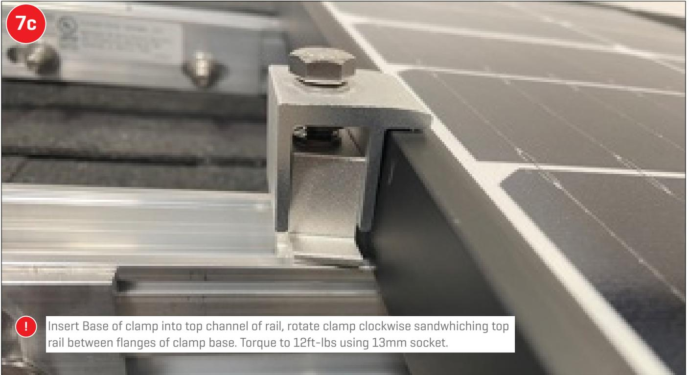
Insert Base of clamp into top channel of rail, rotate clamp clockwise sandwiching top rail between flanges of clamp base. Torque to 12ft-lbs using 13mm socket.
