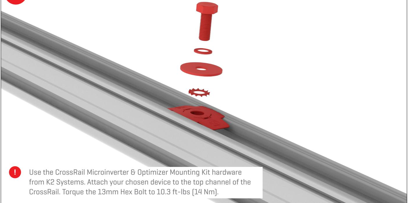
! Use the CrossRail Microinverter & Optimizer Mounting Kit hardware from K2 Systems. Attach your chosen device to the top channel of the CrossRail. Torque the 13mm Hex Bolt to 10.3 ft-lbs [14 Nm].
