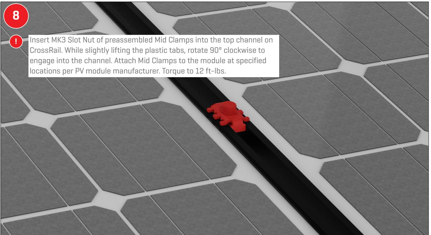
Insert MK3 Slot Nut of preassembled Mid Clamps into the top channel on CrossRail. While slightly lifting the plastic tabs, rotate 90° clockwise to engage into the channel. Attach Mid Clamps to the module at specified locations per PV module manufacturer. Torque to 12 ft-lbs.
